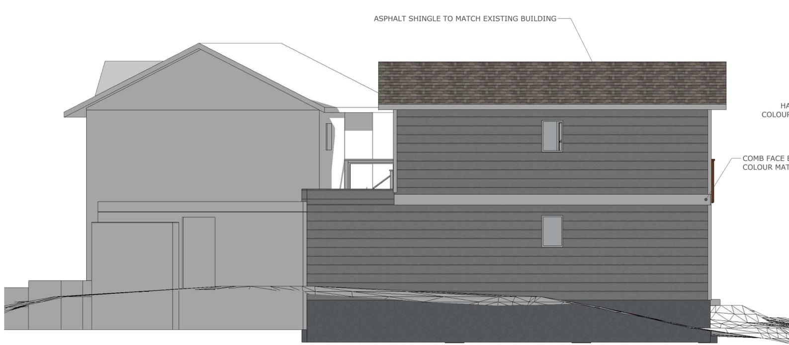
NORTH ELEVATION (SIDE) - SCALE: 1/4" = 1'-0"
